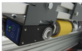
Advanced cutting mark reader
