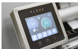
Automatic vertical alignment control panel
