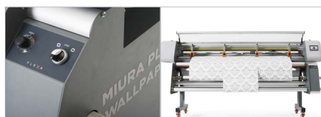
Miura II Plus WP for wallpaper: equipped with front rewinding shafts with independent clutches and speed regulator
